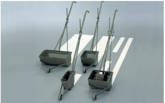
The Borum manual screed boxes can be used for marking one line up to 60 cm (24 inch) or a double line of 10 cm (4 inch) in one run. The thickness of the line can be from 1.5 mm to 5 mm (0.06 to 0.2 inch). Antiskid material can be pre-mixed in order to make the markings less slippery.
