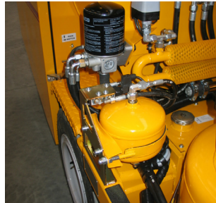
Air drier for bead tank
