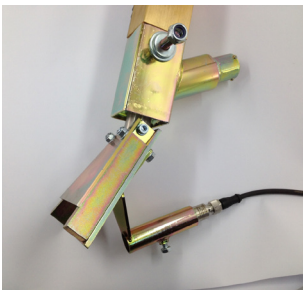
Bead alarm mounted on bead gun
