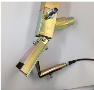
Bead alarm mounted on bead gun
