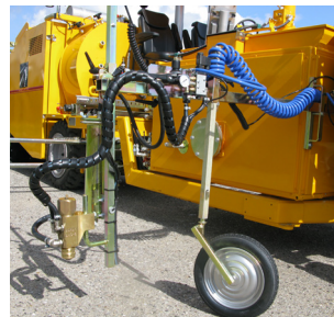
Pre-marking system with paint gun
