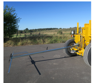
Pointer turning with steering With hydraulic lifting system
