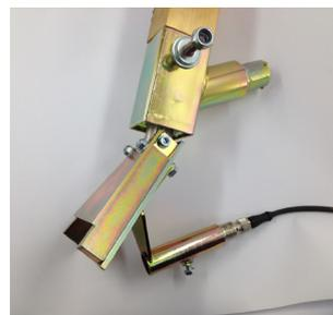
**Bead alarm mounted on bead gun**
