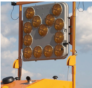
Bar with pneumatic lift for mounting warning lights (Comes without lights)
