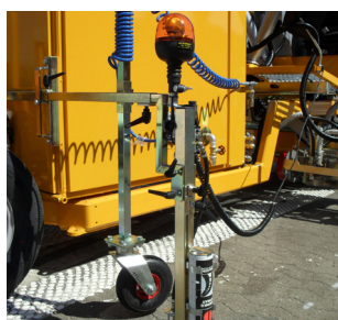
Pre-marking system with paint can
