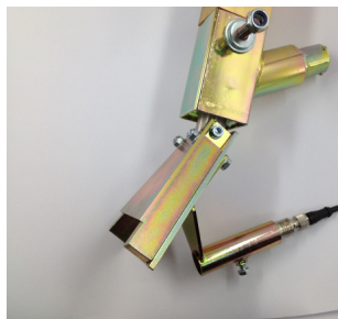
Bead alarm mounted on bead gun
