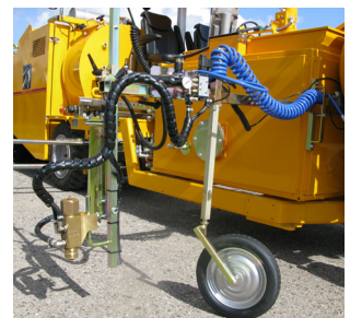
Pre-marking system with paint gun
