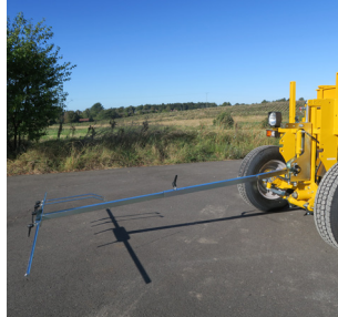
Pointer turning with steering With hydraulic lifting system
