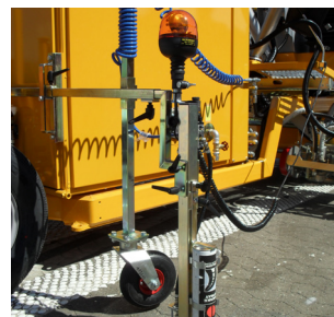
Pre-marking system with paint can
